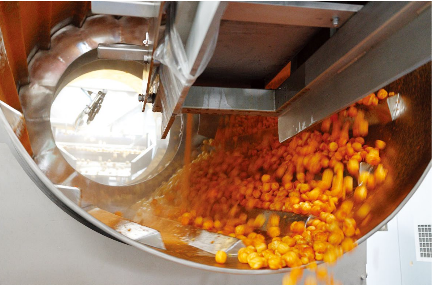
A scene capturing process control on a seasoning line. As the automatically fed extruded snacks dance in the rotating drum, the right amount of oil and seasoning are sprayed at the right time and mixed together.
